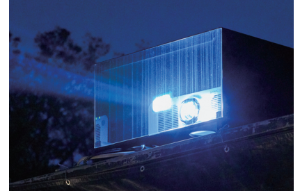
▲ As projection onto the stone rampart surrounding the moat requires a high degree of luminous power, four PT-RZ120JLW units with a brightness of 12000 lm were employed.
